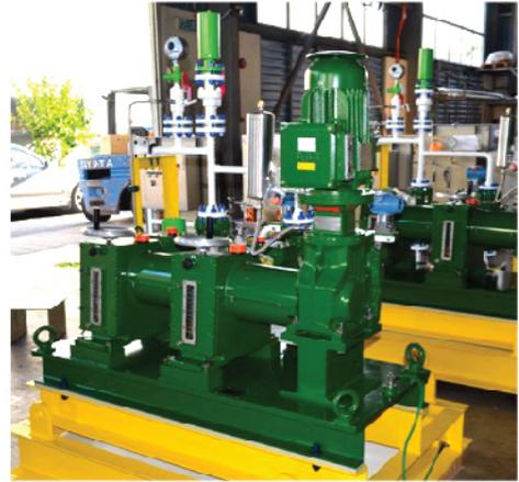
Diesel Injection Skid for Off shore Application
